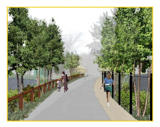
Little Fresh Pond is on the left, Fresh Pond on the right. The Reservoir fence is 5 feet high. The post and rail fence with black PV coated wire mesh, which borders Little Fresh Pond, is designed to stabilize the shoreline by preventing access along its length.
