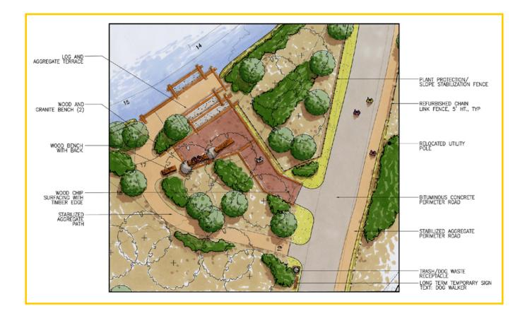
The above drawing is a plan for the southeast access point on Little Fresh Pond. Log and aggregate steps lead up to a viewing platform and down into the water . A wheelchair accessible path, in tan, also leads to the upper level. The darker brown area represents a wood chip path (not wheel-chair accessible) leading to the steps.
